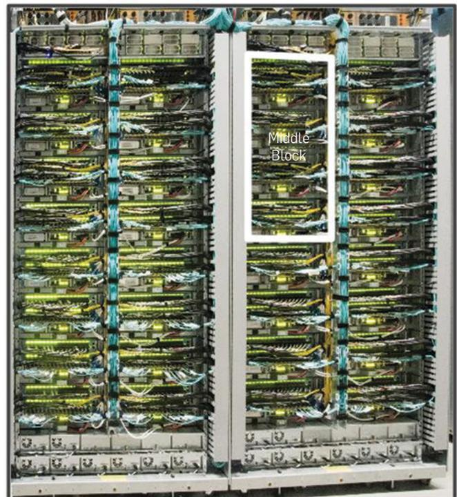
Figure 7. Components of a Saturn fabric. A 24x10G Pluto ToR Switch and a 12-linecard 288x10G Saturn chassis (including logical topology) built from the same switch chip. Four Saturn chassis housed in two racks cabled with fiber (right).
